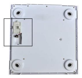
Take battery housing out of scale.
