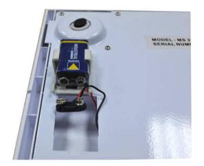
Installing 9V battery
