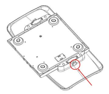
3. Tighten the screw nut on both sides.
