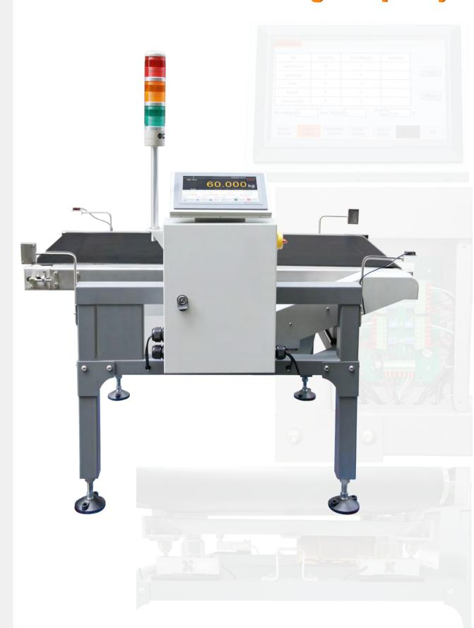
C401A-60K Automatic checkweigher offer a new dynamic weighing technology to solve high-precision problem of a wide range, specially for food, grain, fertilizer, cement and logistics heavy load production lines.
