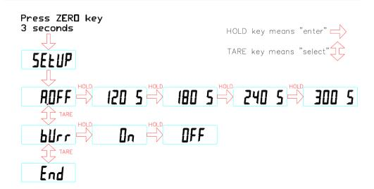
\*\* To apply the changes proceed till END displays on the screen, and then press HOLD to confirm changes.
