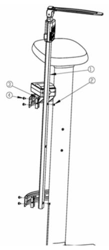
Step 2. Fix HM200D/201D/201M on the bracket and tighten the screw.
