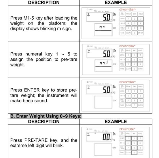
Enter pre-tare weight using 0~9 keys. For example- 5kg.
